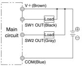
NPN / 1 switch output and 1 analog output
